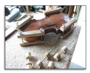
After the glue had dried it was time to clean the neck pocket and neck joint. This involved cleaning the old glue off then gluing and clamping the neck back in, making sure to get the neck angle set properly.
