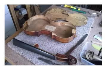
First was to get the soundboard and neck off, done with applications of hot water and palette knives – not for the faint-hearted! I used a hypodermic syringe to get hot water into the neck joint. Fiddles are assembled with hide glue so that they can be taken apart. The glue is applied hot, and heating it loosens it once again.
